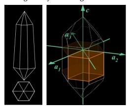
Crystal must be cut so that the tips of both terminations are in perfect alignment with the C-axis (growth axis) of the crystal
